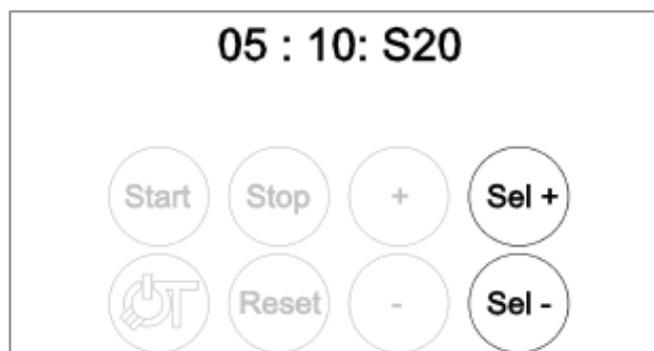
By pressing the keys + and -, you set the desired values of each units of measurement.
