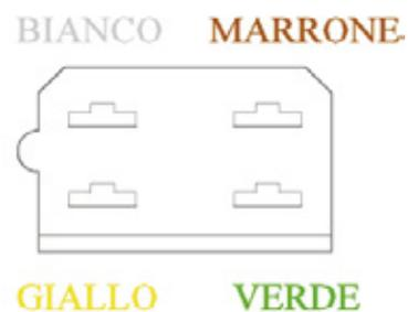
In the package of the TR 400 SERIES, it is enclosed a connector to 4 conductors with Fast-on 6.3mm , for connection to the car system, (The connection will be performed by specialized personnel. Alterations of the original electrical car system could void the warranty of the manufacturer and are thus carried out under the full responsibility of the owner, OnTech will not be held responsible for any malfunctions resulting from these modifications).
