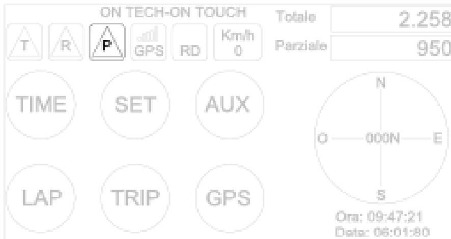
A P inserted in a triangle identifies the sensor of the flow air filter, the signal will come from connecting the wire flow signal " 5" of connector INPUTS to 6 poles supplied and the black wire (GND) connected to the TR module50 ( switch available as an accessory). The activation must be done by connecting the device TR50 to the connector adapter (supplied) in figure "A".
